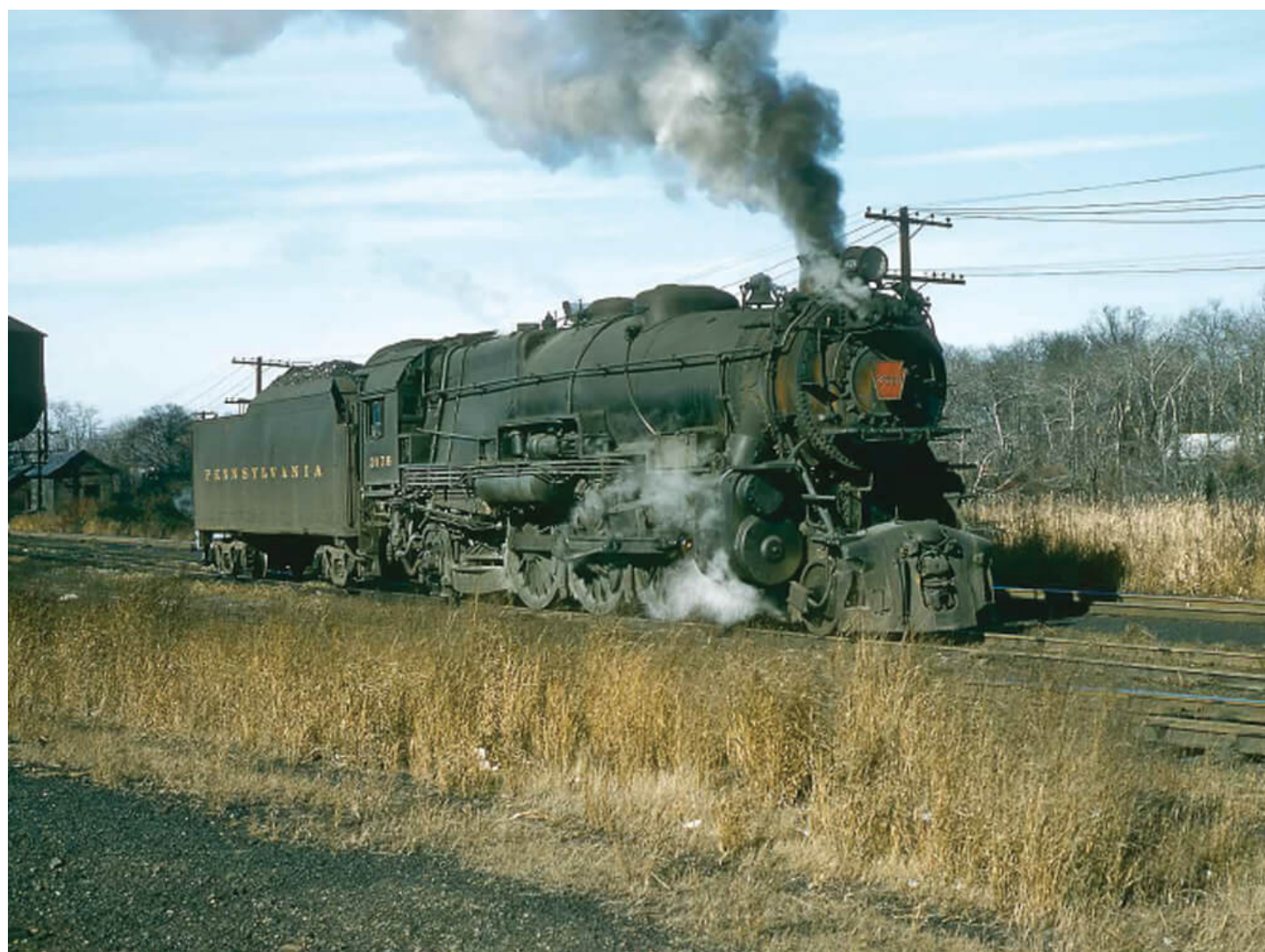
Pennsylvania Railroad 3678, a Class K-4s Pacific (4-6-2) built in 1918 at Pennsy's Juniata Shops, is running light at the New York and Long Branch Railroad's Bay Head Junction, NJ engine terminal on December 1, 1956. Pennsy had 425 of these superb locomotives, designed primarily for passenger service. The New York and Long Branch, a commuter line that operated from South Amboy to Bay Head Junction, NJ, provided their last opportunity to perform. In 1956, 3678 and 19 other K-4s were in the commuter pool at South Amboy. By late 1957, all on-line steam was a memory.
